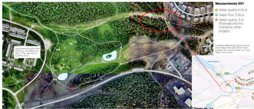
Figure 63 Skellefteå (SE)- Location of water flow and water quality monitors.
