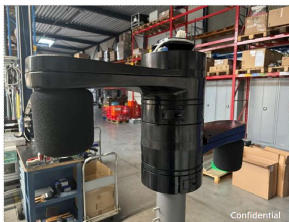
Figure 49: Leuven (BE)- Noise sensor to be integrated in the lighting poles
