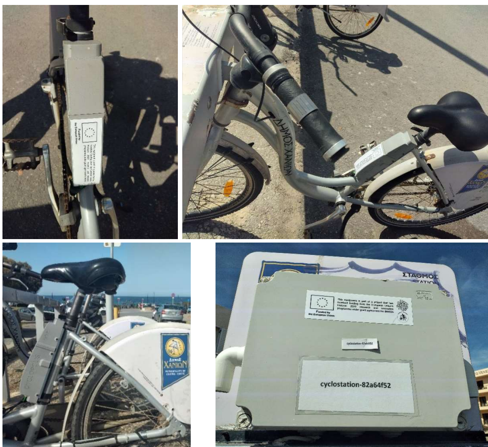
Figure 15: Chania (GR)- Installation of sensors on public bicycles & stations.
